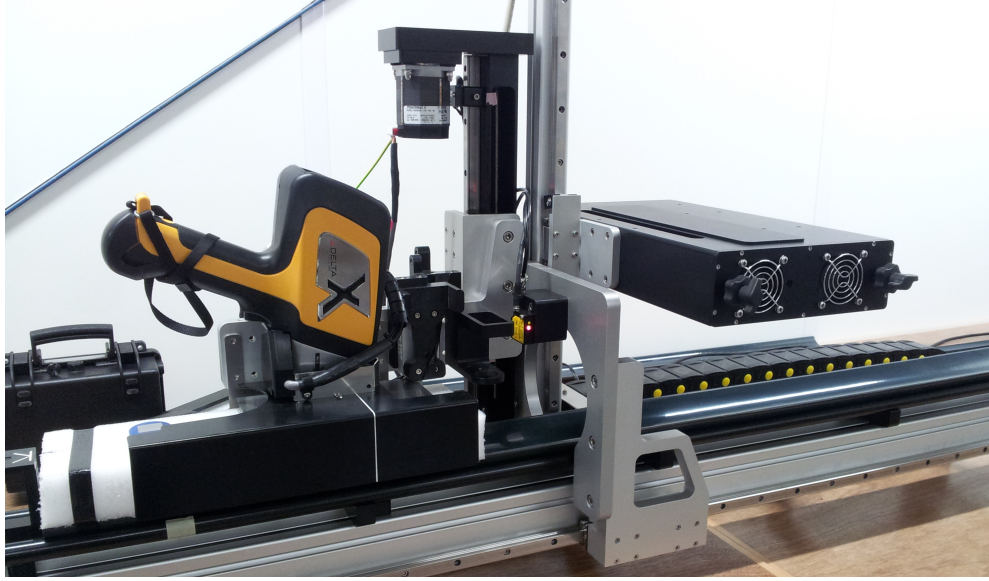
Figure 1: The automated XRF apparatus. A standard hand-held XRF is mounted on a robotic gantry system with laser-guided movement.
